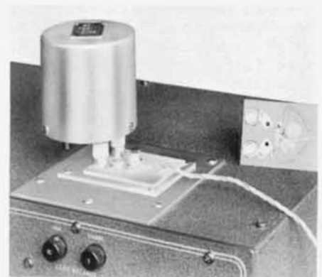
Figure 2. Jig H_{110} , shown, includes binding posts to which the 103-A series coil or other components may be connected for extending the RX Meter capacitance, inductance, or resistance range.
