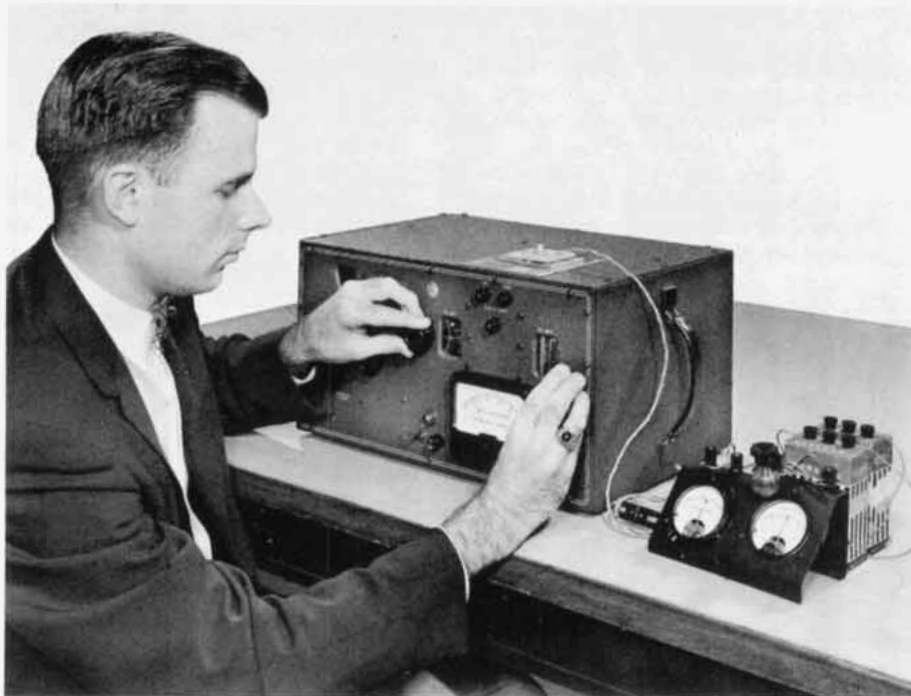
Figure 1. The author is shown measuring a transistor, using the RX Meter, a battery power supply, and a specially made transistor measuring jig.
