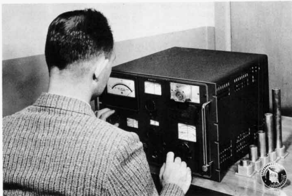
Figure 1. Don Gann, BRC Lab Technician, Checks the 280-A UHF Q Meter with an Impedance Standard
