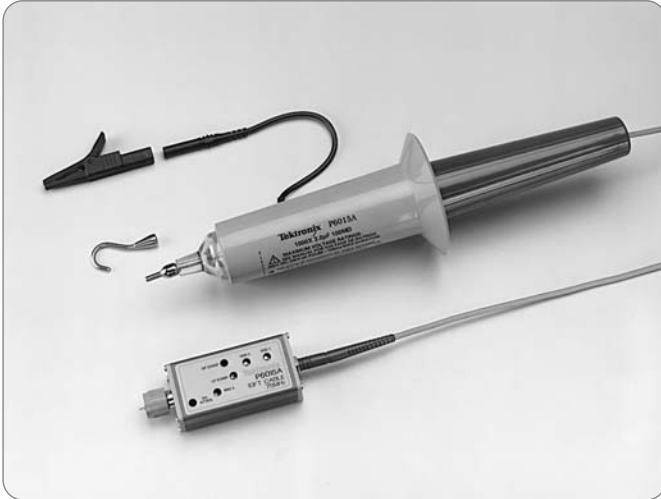
▶ Figure 2-5. The P6015A can measure DC voltages up to 20 kV and pulses up to 40 kV with a bandwidth of 75 MHz.
