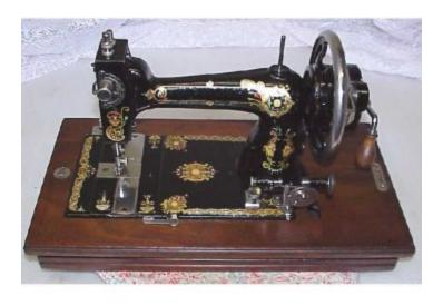
White Peerless 3/4 size hand crank. These lovely little VS machines came in three generations of models, varrying by the tension sysem and the hand crank installation. This is the last version, with the same tension system as the final version of the White VS full size and the White FR. Uses the saame odd bobbin with the shaft in it that the VS does.
