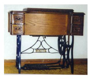
This is the most common White FR treadle cabinet. This one has been refinished. Normally, the word "White" is spelled out in twig shapes pieces of wood on the front panel. Commonly, pieces of this are broken or missing. This is often referred to as the
