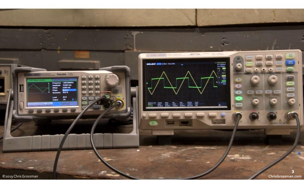
Fast (3ns) rise-time waveform with & without a 50  $\Omega$  feed-through termination on the oscilloscope
