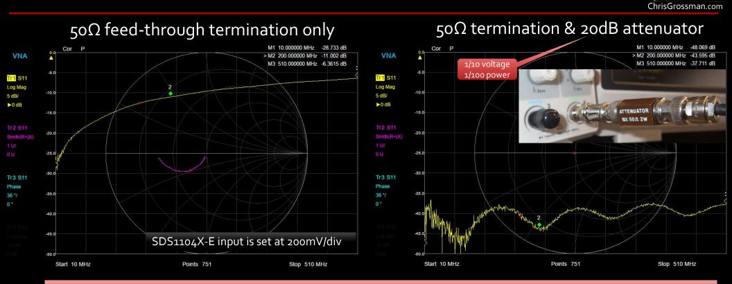
Use of an inline attenuator yields a better match but with a loss of signal magnitude
