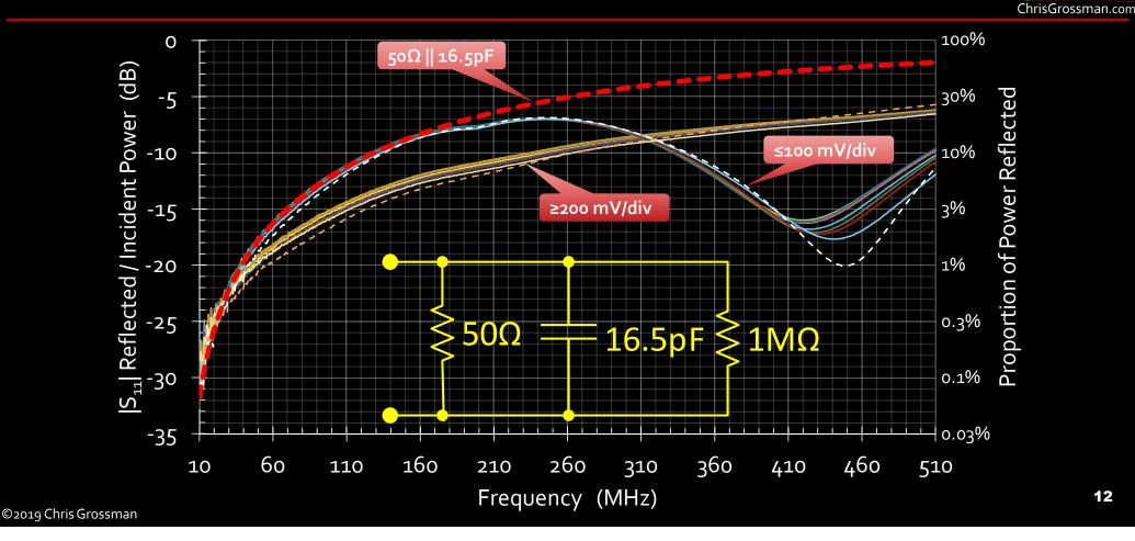
Improve your scope's input match with the use of an attenuator and a feed-through terminator
