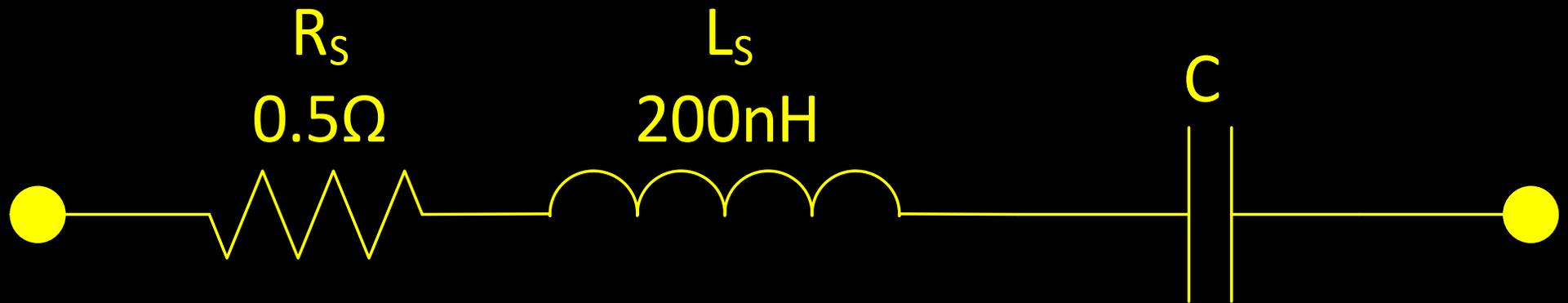
This is the circuit at the terminal posts. Any leads used to connect this to a circuit will have additional inductance.
