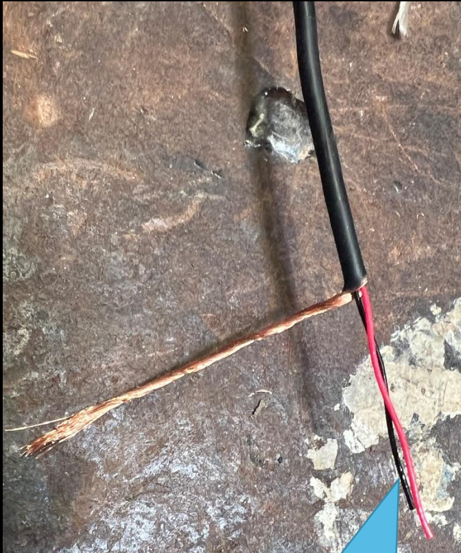
Strip the black wire and combine it with the shield
