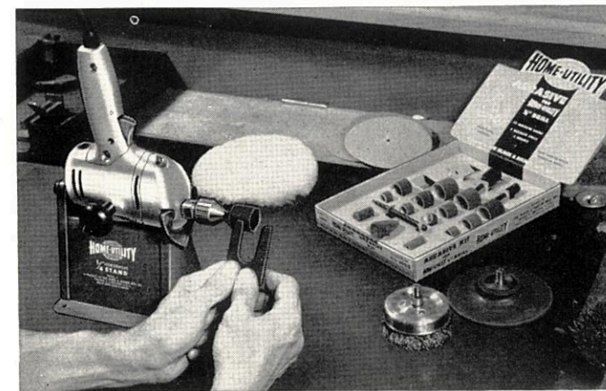
Sander-Polisher in Horizontal Stand using Abrasive Kit
