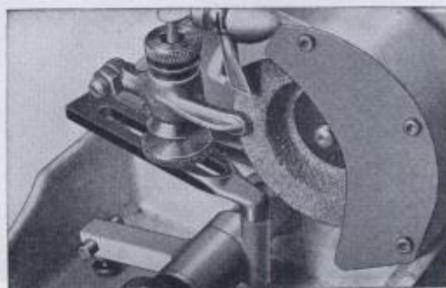
ROCKER ARM GRINDING
