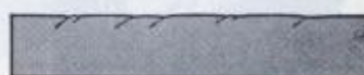
Car Surface After Vitri-Glaze— Peaks Folded Over Into Valleys To Give Smooth, Glazed Surface
