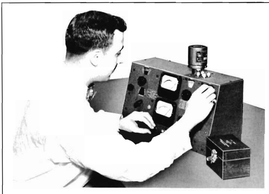
Figure 1. The importance of the quantity Q in the analysis of electronic circuits and components has made the Q Meter a familiar laboratory tool. Here, H. J. Lang, BRC Sales Engineer, is checking the accuracy of a Q Meter Type 260-A with the new Q-Standard.
