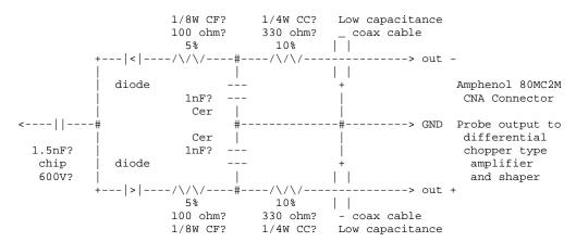
Unmarked diodes are Germanium or Germanium Schottky or Zero Bias Silicon Schottky. They exhibit a sqare-law characteristic similar to point-contact germanium diodes.
