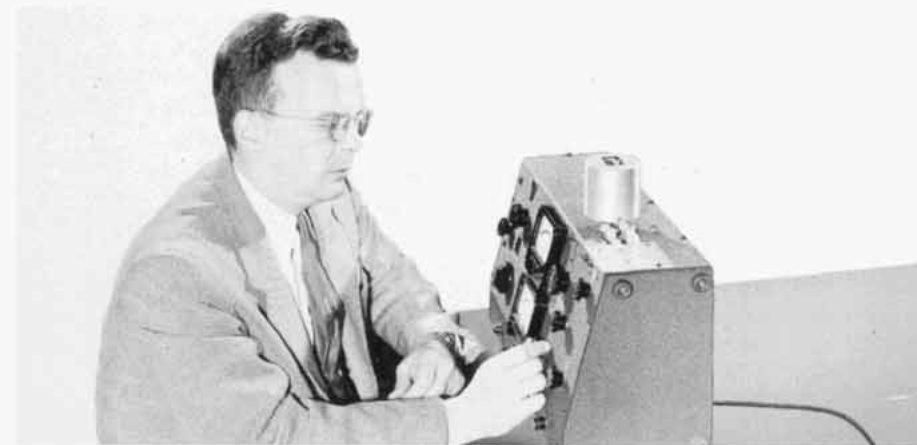
Figure 1. The author measuring the dissipation factor of Teflon.
