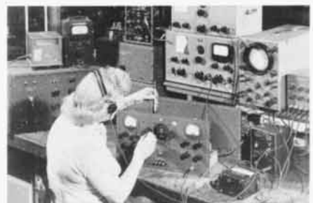
Inspector aligning the RF section of Signal Generator Type 211-A to track with the frequency dial.
