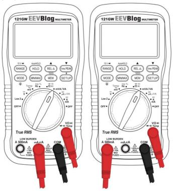
Power measurements require measurements of both voltage and current, be careful to connect the system in a manner that the common terminal is common for both the voltage measurement and the current measurement.
