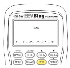
Logged data is stored to an internal Micro SD card which is accessible behind the battery cover. Data is by default recorded once per second.
