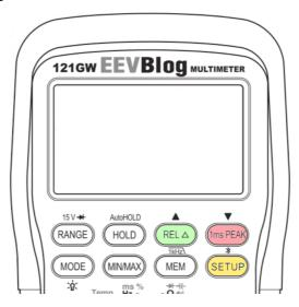
To configure and read settings for the multimeter you can press the *SETUP* button to view the settings. If you press the setup button multiple times you will cycle through the menu, the order of the menu is as follows:
