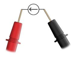
When measuring current be sure to have the leads connected as above and in the correct range, for higher currents ensure that the red lead is connected to the A 500 mA socket.
