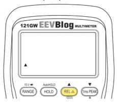
If you are measuring something relative to another measurement or need to calibrate any non-zero error out you can press the *REL* button to zero, the currently displayed value.
