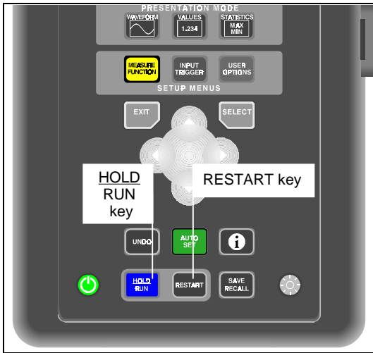
Figure 15 Measurement Control Keys.
