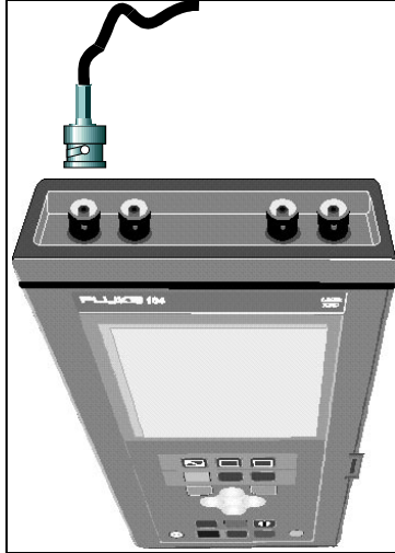
Figure 19 Connect the signal to Input-A.
