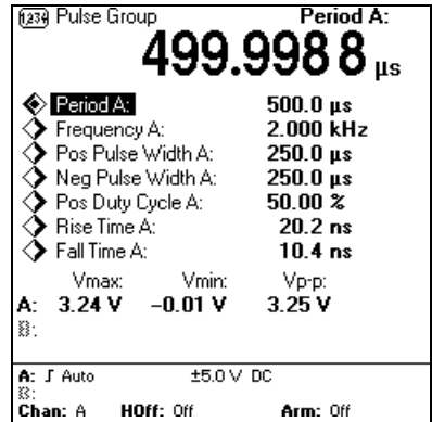
Figure 25 The VALUES screen for Pulse Signal type.
