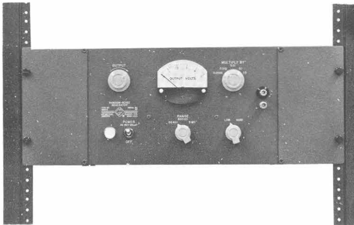
Figure 1. Type 1390-B Random-Noise Generator. (See Section 3 for different mounting arrangements). View at lower right shows Type 1390-P2 Pink-Noise Filter mounted on the generator.
