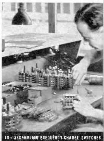
18 - ASSEMBLING FREQUENCY-CHANGE SWITCHES
