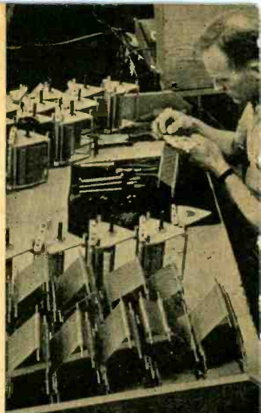
21 - ASSEMBLING OSCILLATOR TUNING CONDENSER
