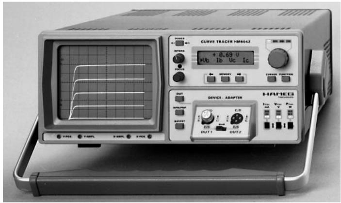
The **HM6042 Curve Tracer** is used to accurately display the characteristics of two and three terminal semiconductor devices. The instrument combines ease of operation and versatile features at an affordable price. Unlike its counterpart, the HM8042 plug-in unit, it uses a built-in **CRT** and an **LCD** to display the characteristics of the device under test.
