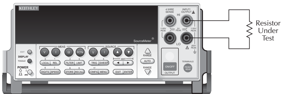
Figure 8-2 Connections for voltage coefficient tests
