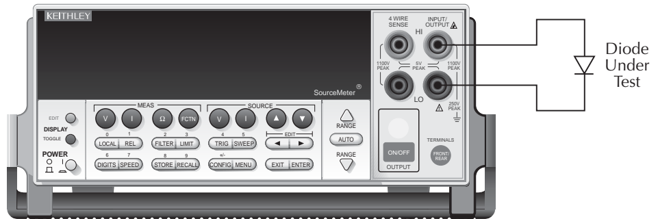
Figure 10-8 Connections for diode I-V tests
