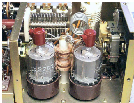
The heart of the PA stage 2 x chunky 6146B tubes
