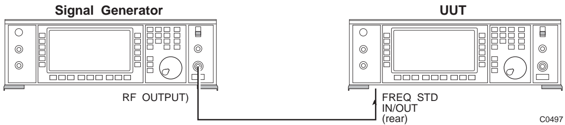
Fig. A-25 Frequency standard locking test set-up
