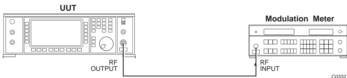
Fig. 5-1-9 Internal AM depth and distortion test set-up
