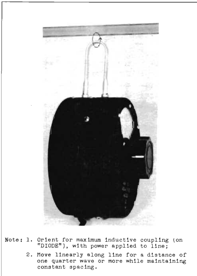
Figure 10 - CHECKING FOR STANDING WAVES ON TRANSMISSION LINES
