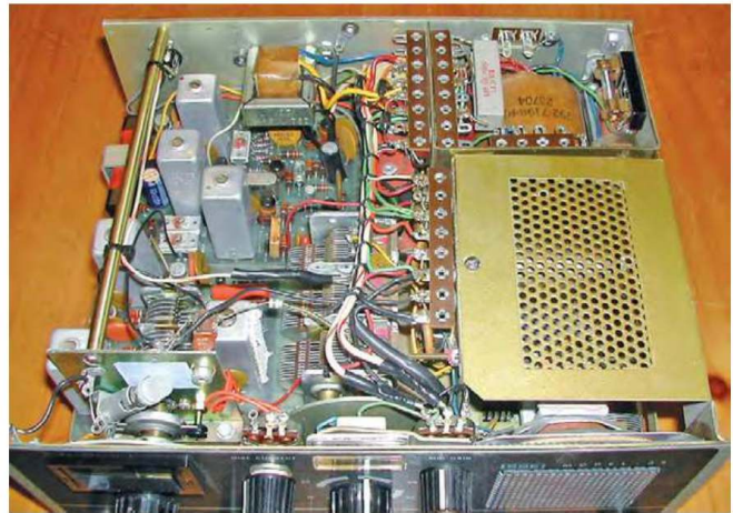
Figure 4 — An inside look of the SB-34 after restoration. [Dale Parfitt, W4OP, photo]
