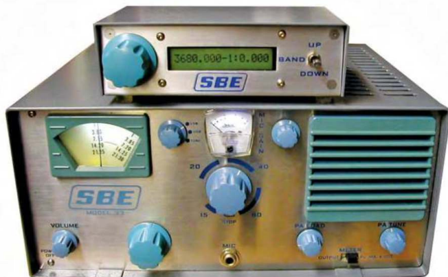
Figure 1 — A restored SideBand Engineers (SBE) model SB-33 with a companion digital VFO. [Dale Parfitt, W4OP, photo]
