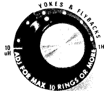
Fig. 22 — The IMPEDANCE MATCH switch is divided into two sections, the four positions in red for TV yokes and flybacks, or all six positions for other type coils and transformers.
