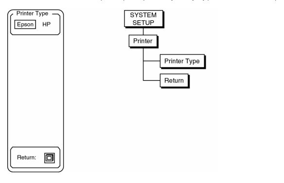
**Printer Type** This function toggles the Printer Type between Epson and HP. Epson is used for any Epson compatible graphics dot matrix printer and HP is used for an HP LaserJet laser printer or compatible.
