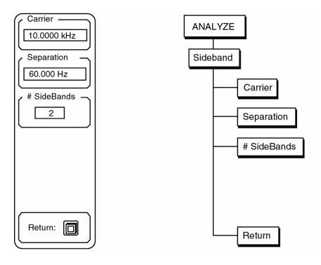
Sidebands are identified according to the formula Sideband  $n = Carrier \pm n$ •Separation where n varies from 1 to the # of sidebands.
