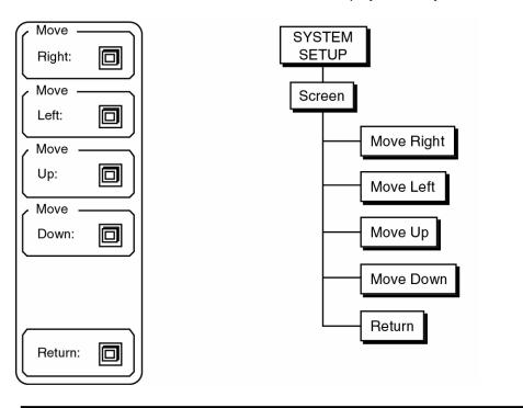
The screen position is stored in non-volatile memory and is retained when the power is turned off. To restore the screen to the default position, power the unit on with the [<-} (backspace) key pressed.
