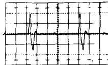
TP(AD), 1V/CM Pulse Xfmr. Input
