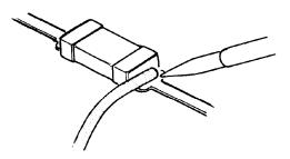
□ Grasp the chip on both sides with tweezers, and gently twist the tweezers back and forth (to break the adhesive bond) while alternately heating each electrode. Be careful to avoid peeling the foil traces from the board. Dispose of the chip when removed.
