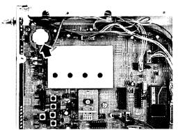
Slide battery downward through slot, then inward and release
